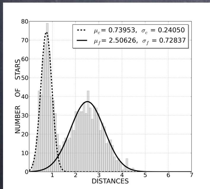
Distance distribution can be approached by a mixture of two 1-D gaussians
