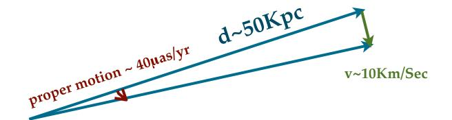
ASTROMETRY of internal proper motions in: p.m. (mas/yr) = v(km/sec)/d (Kpc) \* 0.206265
