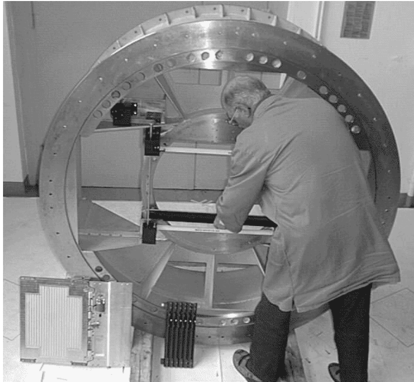
Figure 2. The 1.5m diameter housing structure during a test assembly of the main units: the two storage magazines (to be inserted into the big shaft at left and hidden right), the filter exchange unit with the exchange carriage and a 420 \times 320 \text{mm}^2 dummy-filter (at bottom left).
