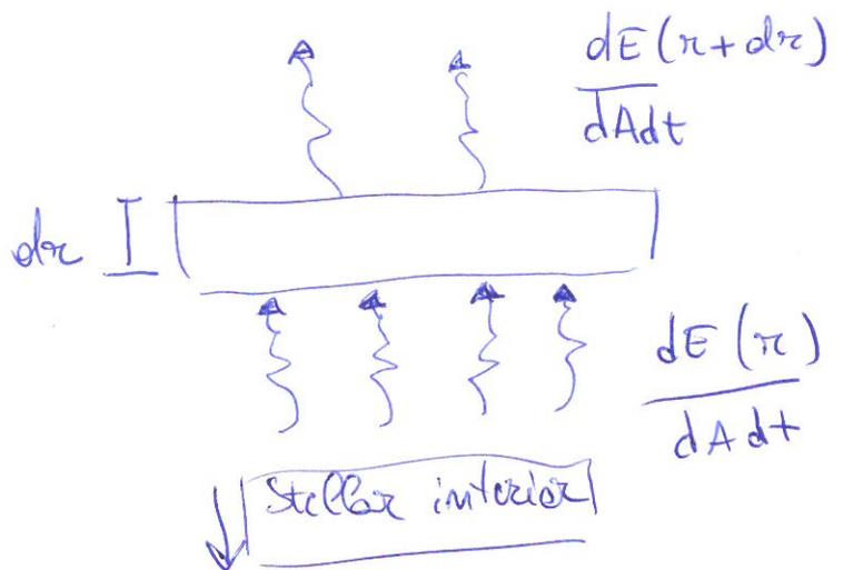
Energy absorbed in the slab per unit area and time
